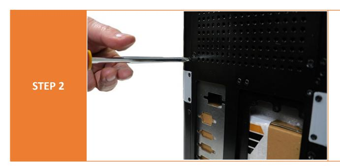
Unscrew the 3 aesthetic skins – screws are at the back of the case.
