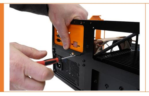
Screw the 3D back panel with screws provided in the bag « screws ».
