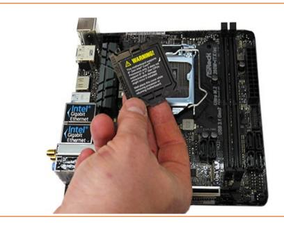
Prepare your motherboard. Remove the plastic protection on the CPU slot.
