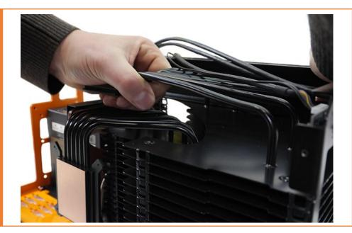
If your components require an assembly with a riser, bend a little bit the GPU pipes to allow more space between the graphic card PCIe port and the mortherboard PCIe slot. Pipes are flexible and easy to bend without risks to breake them when done carefully.
