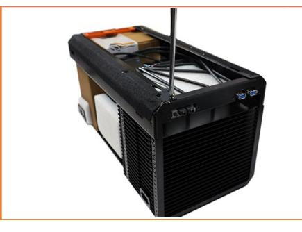
Remove the adhesive taps on the metal stud between GPU cooler and CPU cooler. Reserve if you want to place it back. The adhesive taps are used to prevent scratches during transport. Unscrew the 5 screws on the metal stud.
