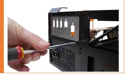
Place your First horizontally, CPU cooler face up. If you plan to change your standard back panel with a 3D printed back panel (customized), start to unscrew the back panel already mounted on The First.
