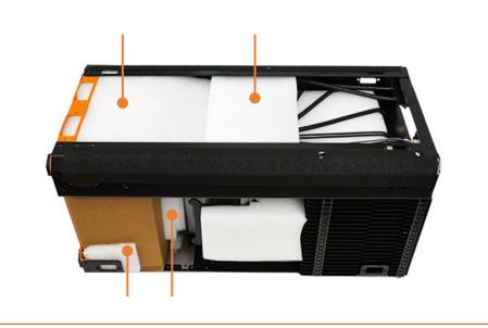
Place The First horizontally with the GPU cooler face up and remove accessible foams.
