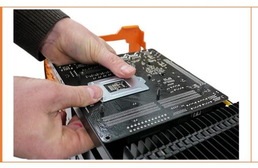
Mount your motherboard for a trial assembly (no thermal grease). Do not hesitate to put some pressure to complete the assembly of the 4 columns into holes.
