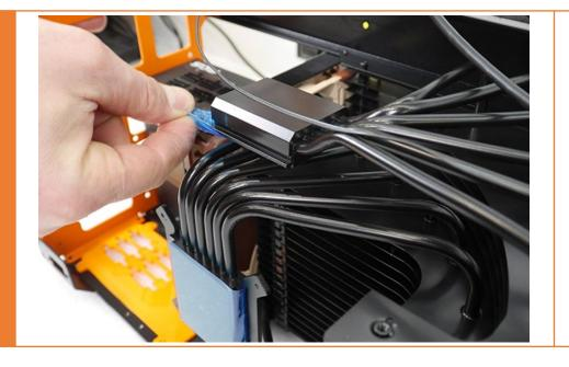
Remove carefully the blue plastic film used to protect the GPU and the CPU cooler blocks.
