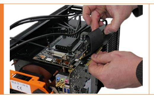
Place your First GPU cooler face up. Verify how you will need to mount your riser for your final assembly. Remove the cards then.
