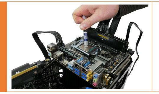
Place your case with the CPU cooler block face up. Place a protection on the heatsink of The First and put your motherboard on it. This will be easier to wired all cables. Put thermal grease on the processor.
