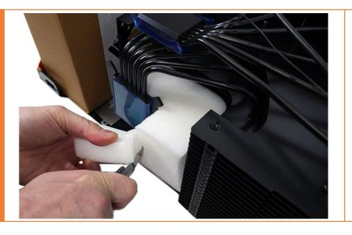
Remove carefully the foams that protect the CPU cooler and GPU cooler.
