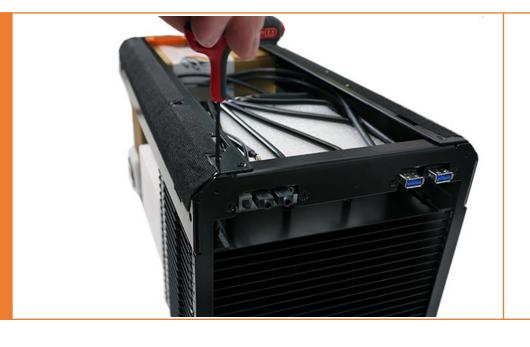
Remove the 2 screws that fix the metal stud onto the heatsink – wrench is required.
