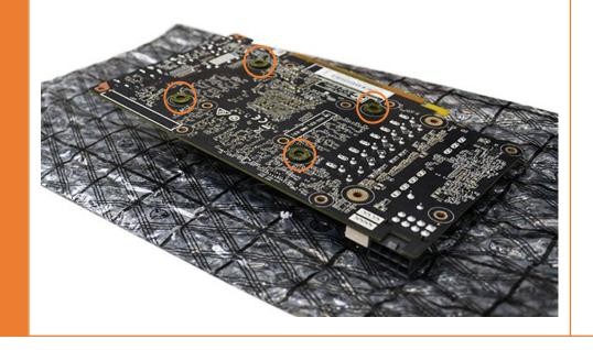
Start to prepare your card with the kit provided in the bag « GPU ». Carefully clean up the area around holes for the fixture mouting (checked on step 26) with alcohol cleaner and stick the plastic washers. Washers have double-face adhesive.
