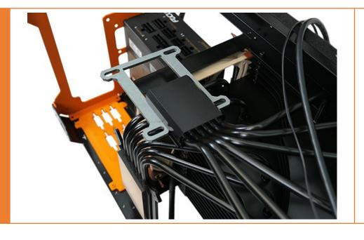
Place your First horizontally, GPU cooler face up. Place the fixture for your graphic card on the GPU cooler block. For some PCBs, the fixture might be mounted from the right to the left.
