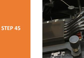
If ordered, mount the VRM cooling or heatsinks provided in our kit of heatsinks and cover VRM and/or memories. Do not forget to clean up VRMs and memories with alchohol cleaner first.
