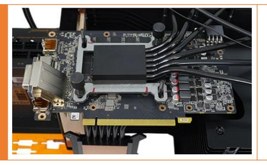
Proceed in a trial assembly (no thermal grease) to check the position of the card, chip, fixture and cooler block. Protect the back of the PCB with a fabric or foam. Use the bag « GPU » and mount the columns, place the spacers, place the springs and place the bars. Do not tight yet. You can also note the position of screws and cooler block on the fixture to help you during the final assembly.
