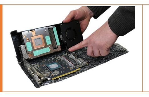
Pay attention to the cable that connect the fan(s) to the PCB. Unplugged carefully.
