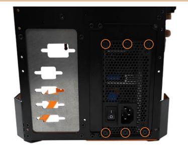
If you mount a SFX power supply, simply screw it on the dedicated part at the back of the case. Screws are provided in the bag « screws ».
