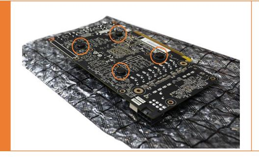
Mount the counternuts, previously cleaned up with alcohol cleaner, into the holes — they should stick to the washer.
