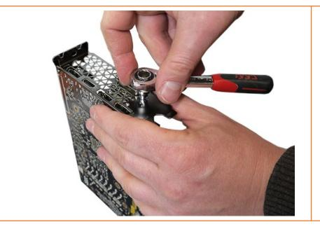
Port panel might need to be removed. If necessary, remove it.
