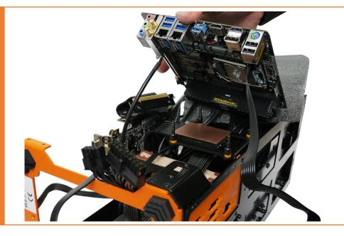
Mount your mortherboard as proceeded during the trial assembly. Place all cables coming from the motherboard behind the CPU cooler block (power switch, SATA cables, USB front panel cable, 24 pin power supply, and sometimes, audio cable). Do not hesitate to put pressure onto the motherboard to make the right contact between the processor and the cooler block.
