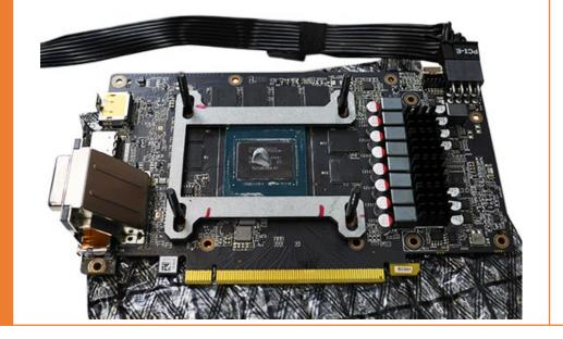
Prepare your graphic card. Connect power cables and apply thermal grease. For full lenght PCBs, you will need to remove columns and fixture to correctly mount your graphic card onto the cooler block.
