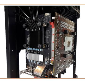
If you do not use a riser, the two cards must be pluged together via their PCIe port / slot. Aligned if needed by loosen the screws.
