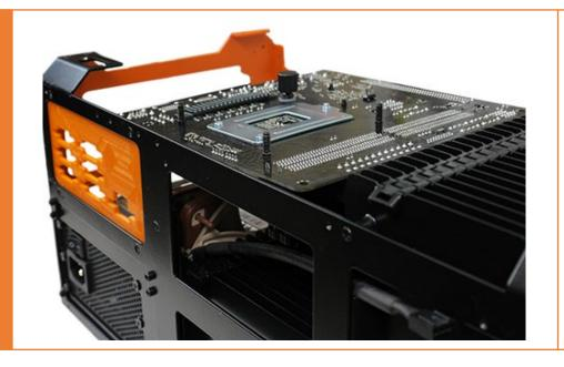
Use spacers and place the bars to complete the trial assembly. Do not tight yet. Check the motherboard is well presed. If not, check no components touche the pipes such as NVMe or heatsinks on the mortheboard. If yes, remove them and use the NVMe slot at the back of the card and use smallers heatsinks available on our eshop.
