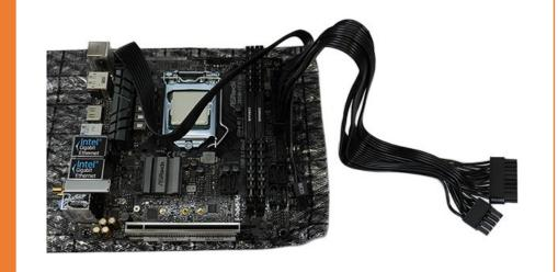
Prepare your motherboard. Prewired with all required cables. Do not forget SSD / HDD cables and do not forget the front panel cables already in place on The First.
