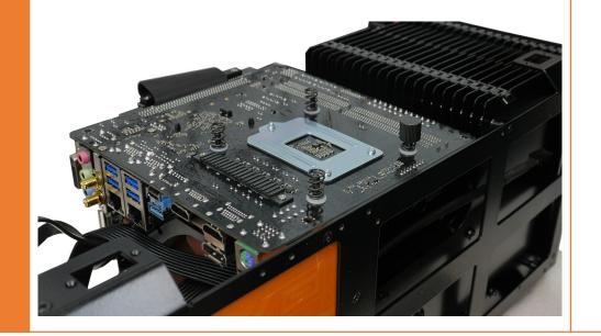
If you do not use a riser, the motherboard and graphic card should be connected together via their PCIe slot / port.
