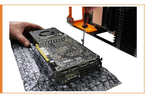
Prepare your graphic card. Remove the fan(s), cooler and back plate if necessary (most of the time). Always protect your card with something between the card and the table.
